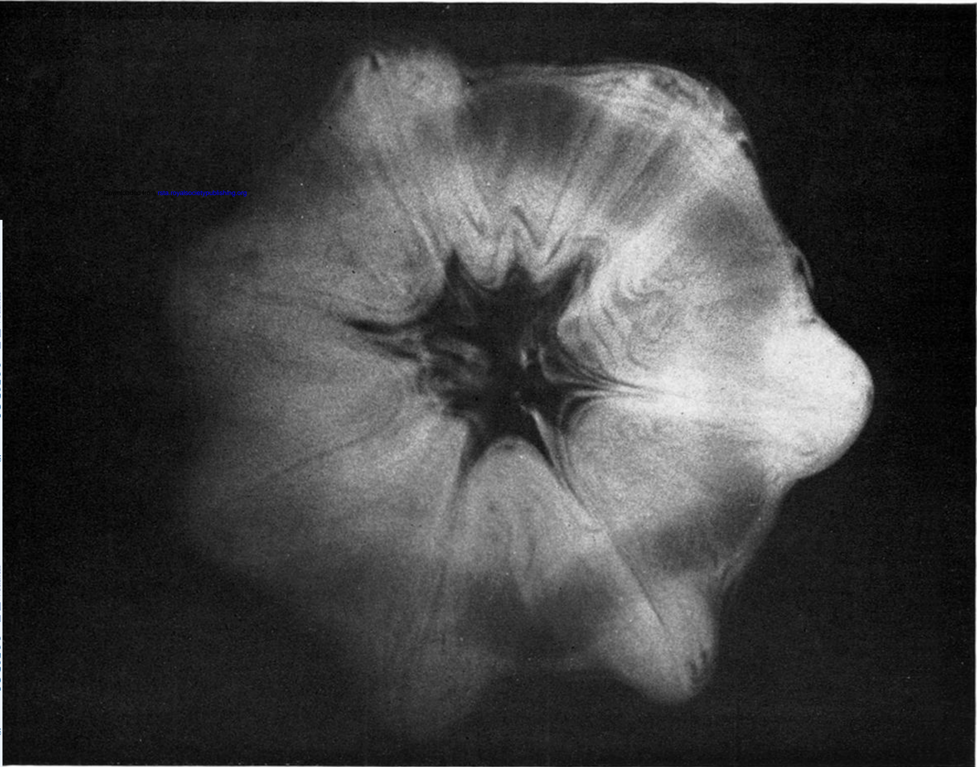
FIGURE 1. Flow visualization of the vortex ring instability; n = 7 . Taken from Widnall & Sullivan (1973).
